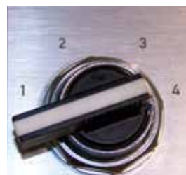
4 Position selector switch located on 2 hand control pedestal.
